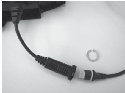
(On Medley with separate power supply) connect the wire from the power supply to the wire from the control unit and secure the connection with the enclosed wire lock
